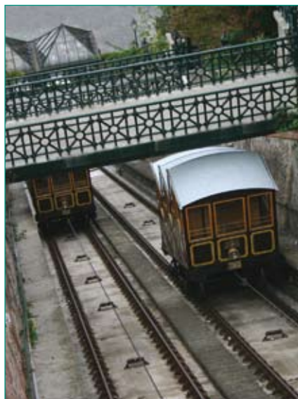
A funicular railway in Budapest, Hungary. It relies on balancing forces.
