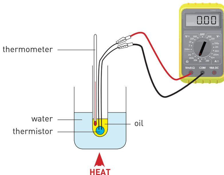
*Note: Cooking oil helps the heat transfer to the thermistor and doesn't conduct electricity.*
