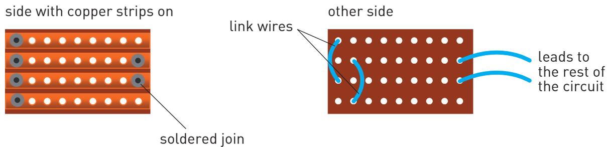
Alternate tracks are joined together with link wires, as shown. Each pair of linked tracks is separated from the other by an insulator, so the resistance between the leads will be very large (more than a million ohms) when the sensor is dry. Moisture will lower the resistance.
