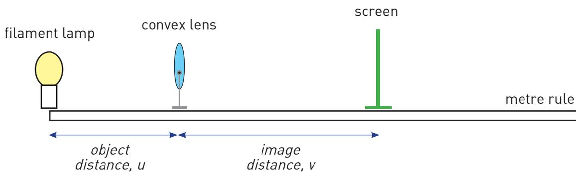
1. Place a bright filament lamp (the *object*) so that the centre of the lamp is level with the 0 cm mark on (or just next to) a metre ruler.
