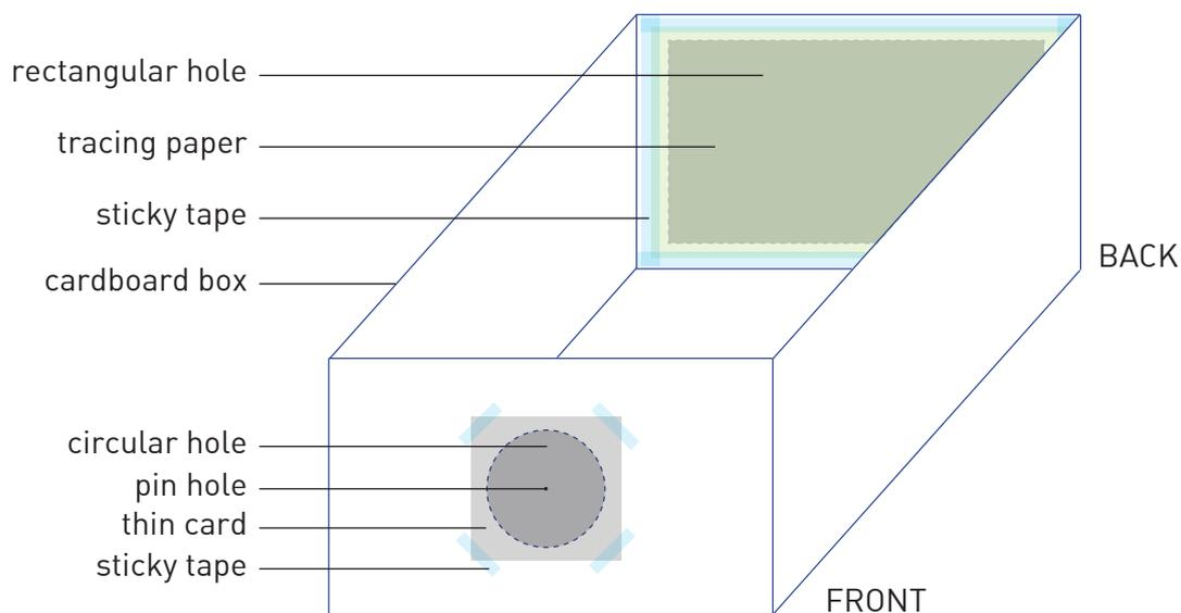
9. Hold the pin hole close to a bright filament bulb. Note what you see on the screen.
